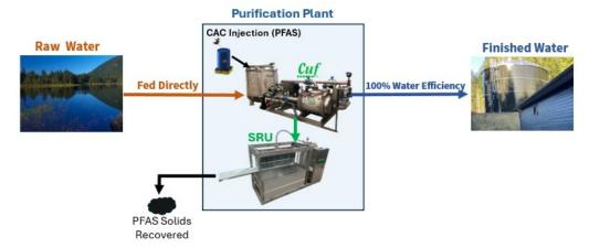
**Cuf** <sup>®</sup> Activated Carbon (**CAC**) is a high-efficiency enhancement that strengthens PFAS removal in both surface water and groundwater. This optional feature complements the core capabilities of the **Cuf** <sup>®</sup> system and can be integrated at any stage, whether during the initial installation or as a future upgrade.
