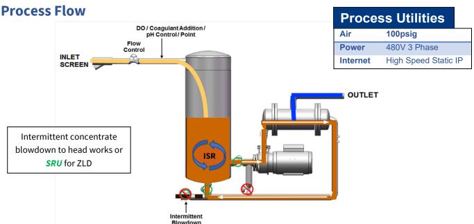
In certain applications dissolved oxygen or a common coagulant is injected to oxidize metals or agglomerate or DOC. These reactions occur in the ISR (In-Situ Reactor). No upstream coagulation basins or clarifiers pretreatment is required, just the *Cuf* platform.
