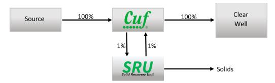
A concentrate blow down is sent to **SRU** (Solid Recovery System) where a 20% solid is achieved without the need for chemical or labor.
