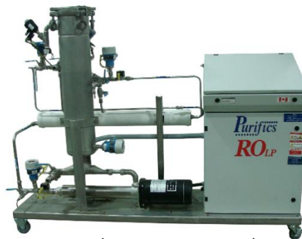
RO (Reverse Osmosis LP)
