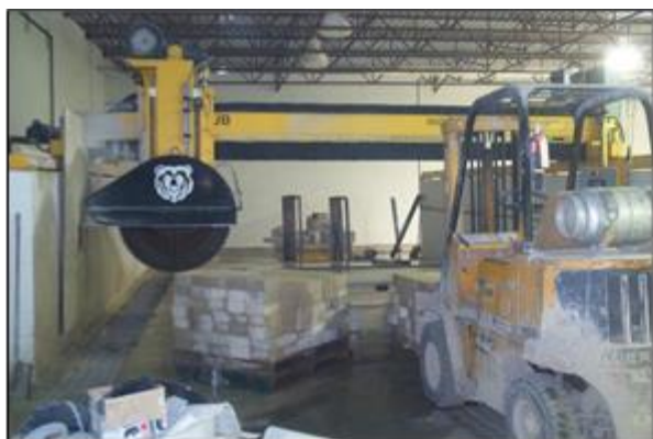
Cutting machinery utilized water for coolant and dust suppressant
